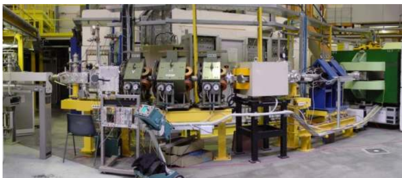
DRAGON at TRIUMF ISAC Used to measure ^{21}\text{Na}(p,\gamma)^{22}\text{Mg}
