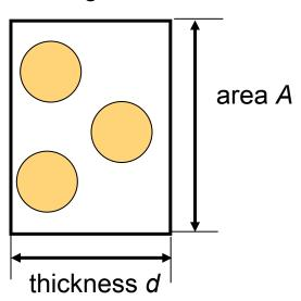
assume thin target (unattenuated beam intensity throughout target)
