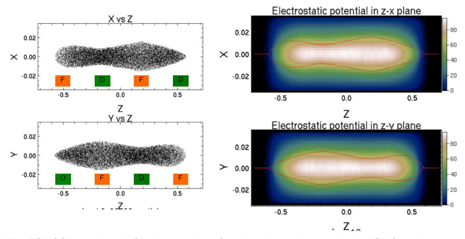
File FODO3D.py - basic 3D simulation of an ion beam in a periodic FODO lattice:
