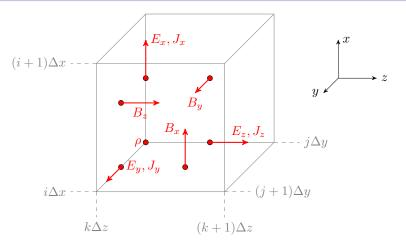
The different components of the different fields are staggered, so that all derivatives in the Maxwell equations are centered (Yee, 1966).
