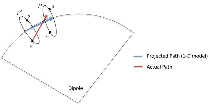
Dispersion in the dipole spreads out the beam in the bending plain
