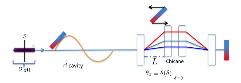
Use acceleration off-crest in the rf cavity to correlate energy with longitudinal position.
