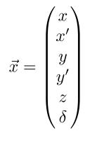
For linear optics, we can use matrices to represent components of an accelerator beamline. This R-matrix transforms the phase space state from initial to final:
