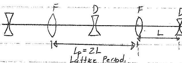
This is the simplest "FODO" alternating gradient lattice?
