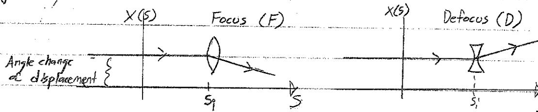
This action can be specified by transfer matrices applied at  $s=s_i$ :
