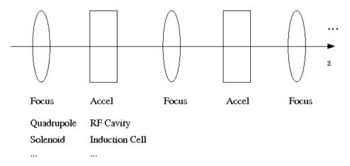
Sometimes functions like bending/focusing are combined into a single element
