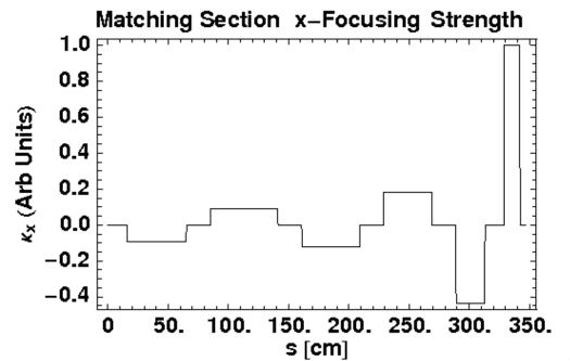
Example corresponds to High Current Experiment Matching Section (hard edge equivalent) at LBNL (2002) Equations presented in this section apply to a single particle moving in a beam under the action of linear applied focusing forces. In the remaining sections, we will (mostly) neglect space-charge ( $\phi \to 0$ ) as is conventional in the standard theory of low-intensity accelerators.
