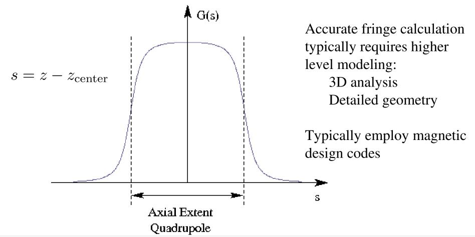
For many applications the actual quadrupole fringe function G(s) is replaced by a simpler function to allow more idealized modeling
