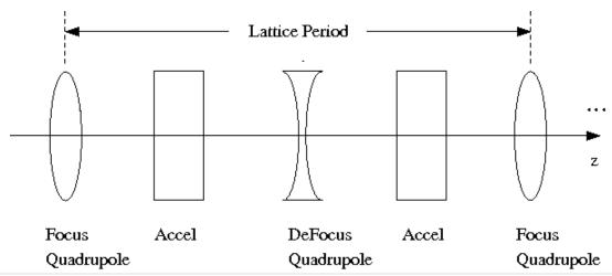
Lattices for rings and some beam insertion/extraction sections also incorporate bends and more complicated periodic structures:
