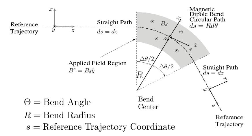
In this perspective, dipoles are adjusted given the design momentum of the reference particle to bend the orbit through a radius R.
