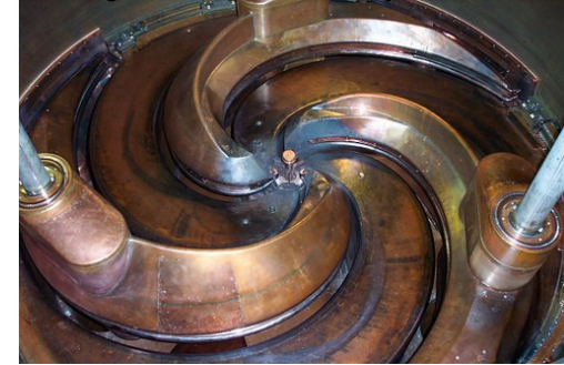
Accelerating "dees" of the K1200 cyclotron
