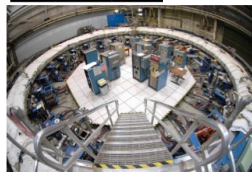
"g-2" storage ring as assembled at Brookhaven National Lab (NY)
