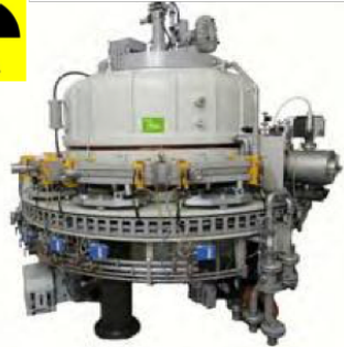
Rhodotron, commercial electron beam accelerator used For sterilization of medical devices
