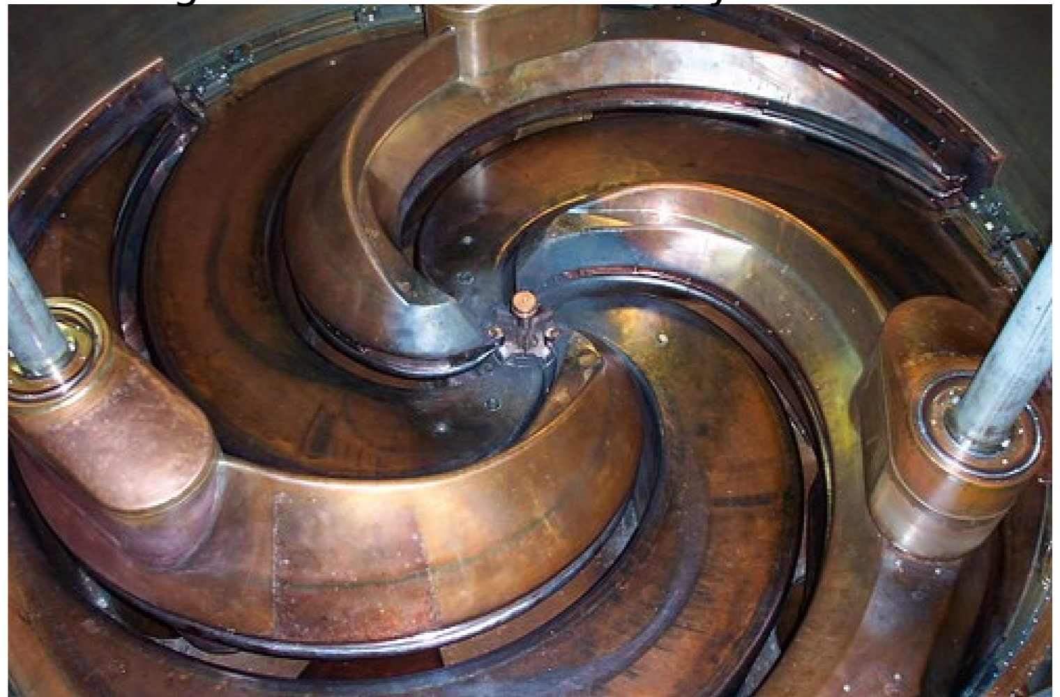
Accelerating "dees" of the K1200 cyclotron
