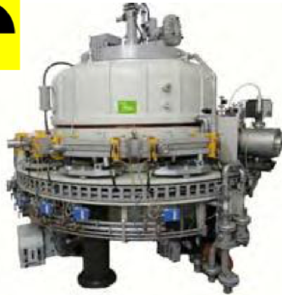
Rhodotron, commercial electron beam accelerator used For sterilization of medical devices
