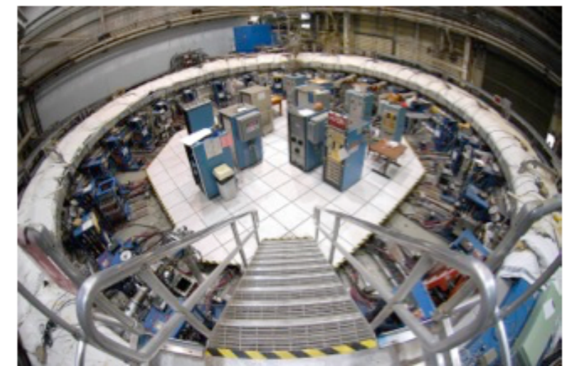
"g-2" storage ring as assembled at Brookhaven National Lab (NY)
